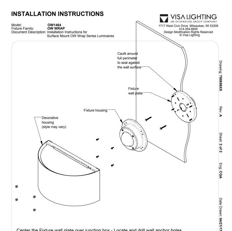
Center the Fixture wall plate over junction box - Locate and drill wall anchor holes.
