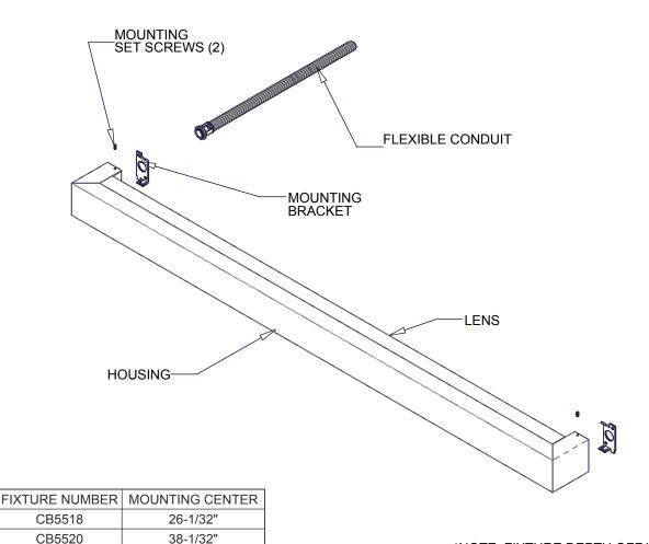
Secure mounting brackets to wall or junction box (JBC option) at mounting center locations, shown on table 1. with hardware (by others). The mounting may be different than what is shown above, depending on which fixture/option is ordered.
