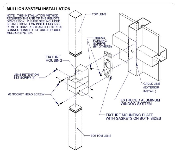
Important: Exterior installation requires caulk along perimeter of housing (or J-Box Cover). SEE SHEET 4.
