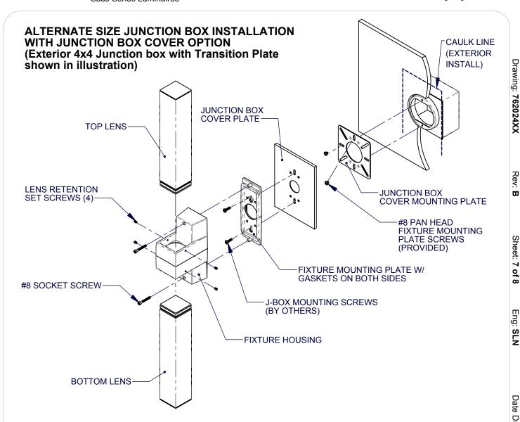
Important: Exterior installation requires caulk along perimeter of housing (or J-Box Cover). SEE SHEET 4.
