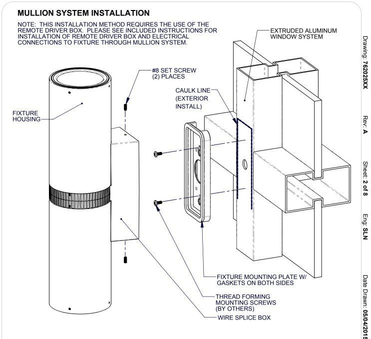
Important: Exterior installation requires caulk along perimeter of housing (or J-Box Cover). SEE SHEET 4.
