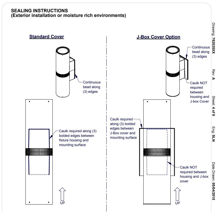
**IMPORTANT**: Caulk must be applied to a clean and dry surface. All surfaces must be free of debris and residue to ensure a watertight seal. Faulty or missing caulk will cause electronic failure.
