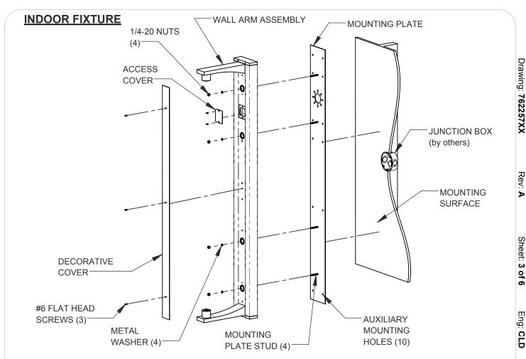
\*NOTE: LAMP HOUSING IS NOT SHOWN (<u>FOR REFERENCE ONLY</u>) TO HELP WITH INSTALLING FIXTURE TO THE WALL.
