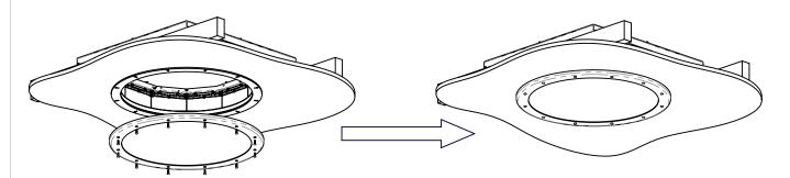
STEP 5: INSTALL LENS ASSEMLY ONTO LENS ANCHOR PLATE
