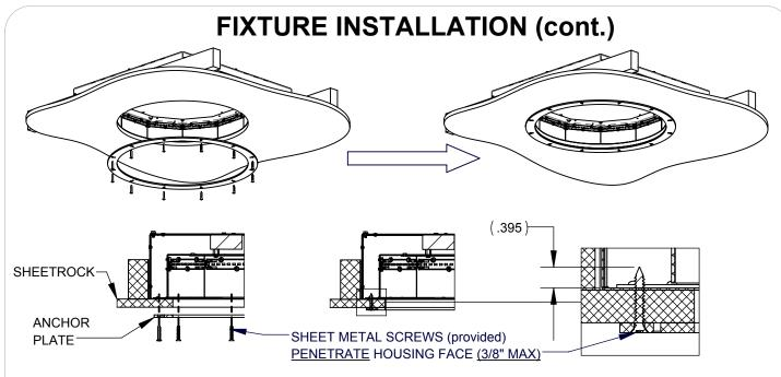
STEP 4: INSTALL SHEET METAL SCREWS (included) THROUGH ANCHOR PLATE, THROUGH SHEETROCK, AND INTO BOTTOM SIDE OF FIXTURE HOUSING
