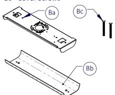
1. Remove the Cover Screws (Bc) holding onto the Cover (Bb). Save for later.
