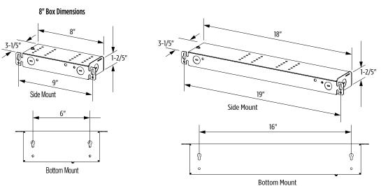
Remote driver boxes have knockouts for conduit connections
