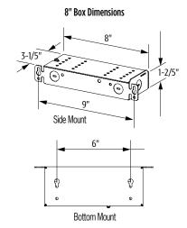
Remote driver boxes have knock-outs for conduit connections
