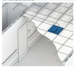
If corridor plenums are overcrowded, the driver can be mounted within the patient room ceiling utilizing the Top Mounted Driver option (TMD). Driver compartment can be accessed via adjacent ceiling tile
