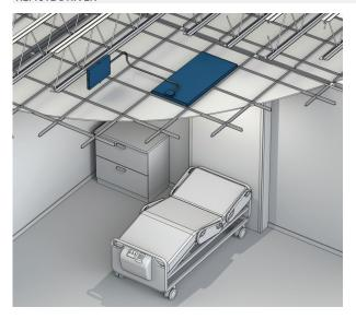
The slim Remote Driver compartment can be mounted in remote locations such as corridors and wiring closets on the floor or wing of the facility using low voltage wiring.
